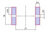
solder stencil recommended stencil thickness 120µm
